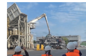
Touring Toyota Metal Co., Ltd. (Participants watch end-of-life vehicles being loaded into a pre-shredder)
