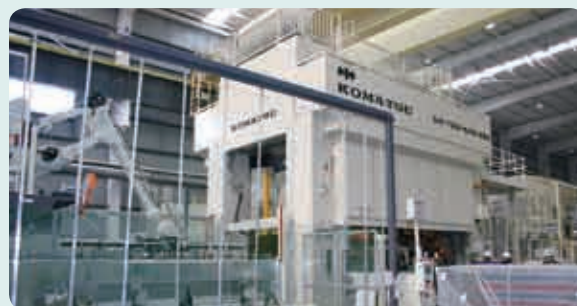
Steel blanking processing equipment (Photo shows facility in Tianjin, China)
