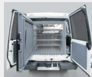
Interior of the vehicle with a dedicated vaccine refrigerator installed
