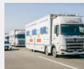
Three large trucks being driven on an expressway at a speed of 80 km/h while maintaining an inter-vehicle distance of approximately nine meters
