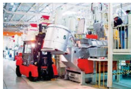
Supplying aluminum in molten form eliminates one melting process.
